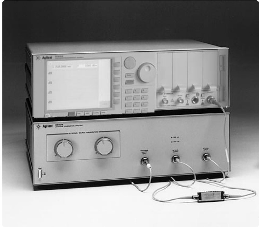
Figure 5. Polarization mode dispersion measurement setup using the Agilent 8509C and Agilent 8164 or Agilent 8168 lightwave sources.
