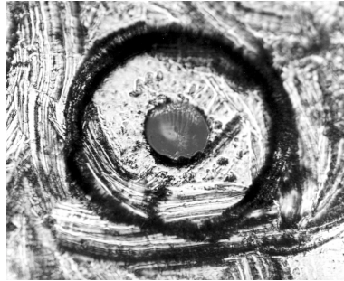
Figure 1-6. Damage from improper cleaning.
