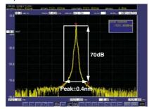
Close-in Dynamic Range 70 dB at peak ±0.4 nm, resolution setting 0.02 nm (typical)
