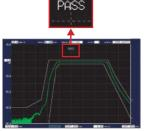
Sample waveform of PASS/FAIL test
